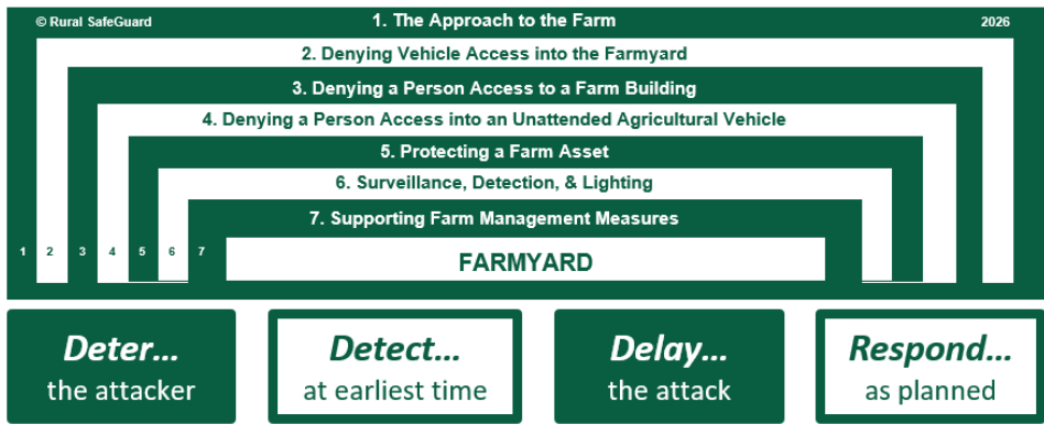
Figure 7: The seven levels of protection model applied to farm security reviews.
